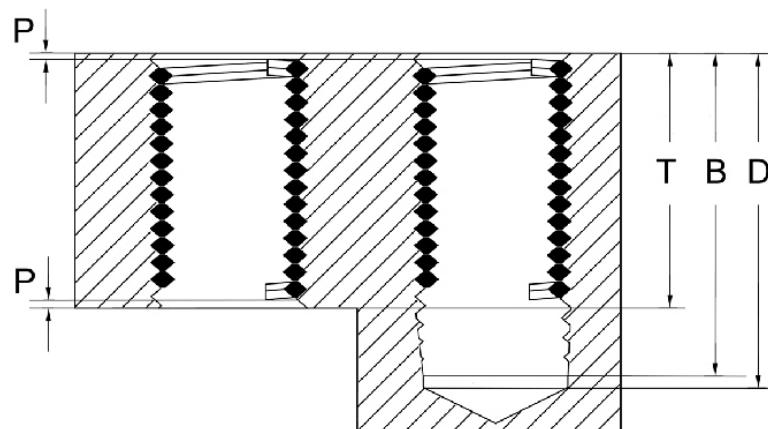
P Installed insert 1/4 – 1/2 pitch below the surface
